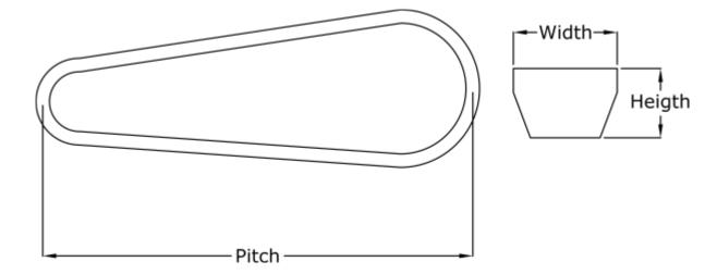
$\begin{array}{ll} \text{Datum Llength} = 5864 \\ \text{Height} & = 10 \\ \text{Length inside} & = 5805 \\ \text{Type} & = BB228 \\ \text{Width} & = 17 \end{array}$
